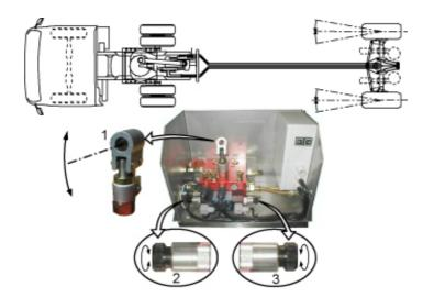
If the electronic system should fail, it is still possible to return the wheels of the trailer to the straightahead position. Follow these steps:
