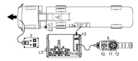
Place the truck in the straight-ahead position in front of the trailer. Indicator lamp (L2) goes on. Continue driving forward slowly and turn the wheels of the trailer using the buttons on the remote control (3), (13) or (9) so that the wheels return to the straight-ahead position.
