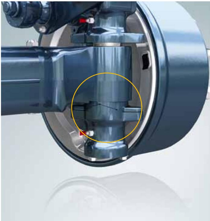
Steering housing when driving straight ahead (zero position).
