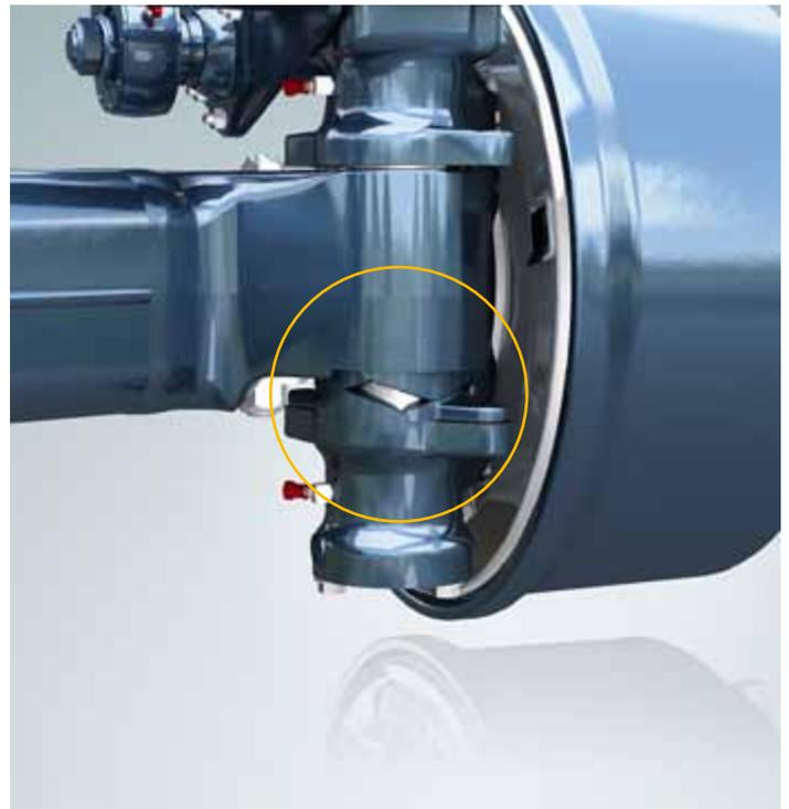
Steering housing when cornering (up to 27 degrees, depending on vehicle model).
