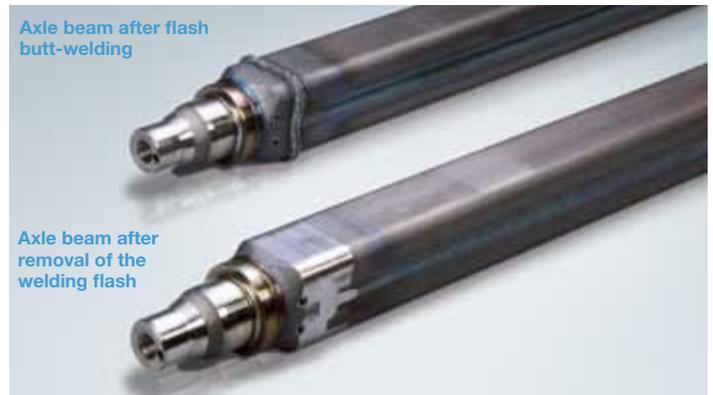
Axle beam after flash butt-welding
