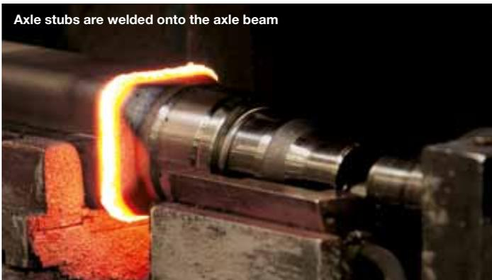
Axle stubs are welded onto the axle beam
