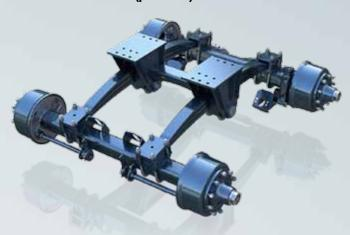
BPW hydro-pneumatic suspension systems (p. 60-61)
