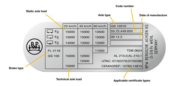
The BPW type designation (see axle type) is composed of a letter group and a number group. The letter group identifies the type of axle and suspension version as well as defining the hub version. The number group specifies the axle load on the ground in kilograms and the number of wheel studs per wheel hub.
