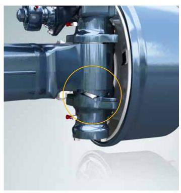
Steering housing when cornering (up to 27 degrees, depending on vehicle model).
