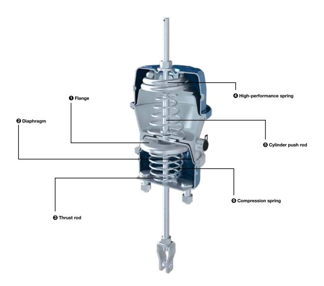
Operation of the service brake: As soon as the compressed air acts on the diaphragm ②, the force generated (area x pressure) acts on the flange ① and the push rod ③. The force is transferred to the wheel brake in accordance with the brake pressure applied. When the brake cylinder is vented, the compression spring ③ moves the flange ① with the push rod ③ and the diaphragm ② back to their original positions.
