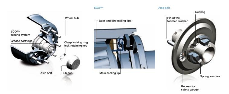
The proven ECO Unit is a master when it comes to ease of maintenance and efficiency. This is not only because of the reduced weight but also, for example, the use of globally available DIN ISO tapered roller bearings as well as rapid removal/installation using the central axle bolt, similar to Formula 1. Innovative design features such as the grease cartridge, the practical bayonet lock for the hub cap and the axle bolt with integrated torque limitation underline BPW's power of innovation.
