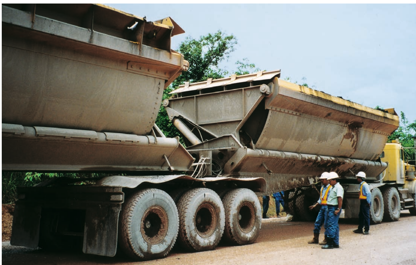
Truck/trailer combination with heavy-duty air suspension
