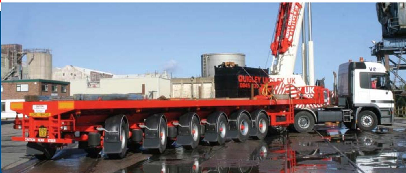
***The hydraulic steering system with steered swivel axles for extendible, tank and rock semi-trailers as well as tippers and ballast trailers***
