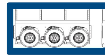
The TRIDEC independent wheel suspension LV-O (non-steered) is an advanced wheel suspension that makes it possible to create more load space in a trailer.
