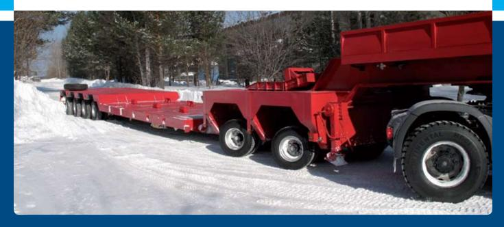
The oscillating axle suspension for extremely heavy transport such as the transport of bridge sections, excavators, etc.
