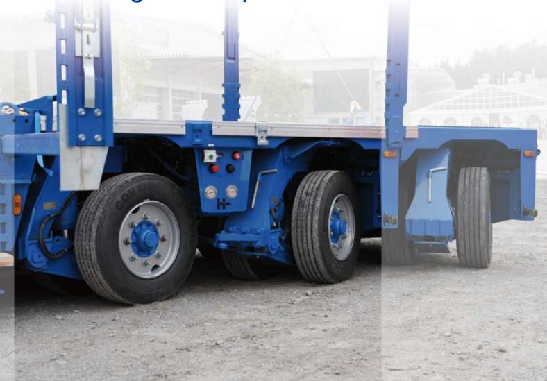
The oscillating axle suspension for extremely heavy transport such as the transport of bridge sections, excavators, etc.
