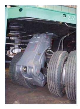
The TRIDEC TP-O oscillating axle suspension has been developed for extremely heavy transport. This oscillating axle suspension can be used in conjunction with the TRIDEC HFE steering system.
