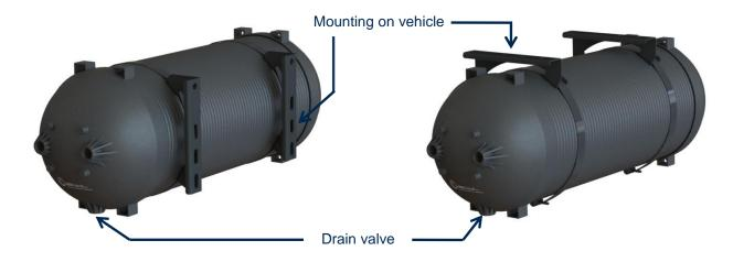
It is important to ensure that the air tank is mounted, as shown above on the vehicle chassis or superstructure. It is recommended that the air tank is mounted in a protected area under the vehicle, e.g. between the longitudinal chassis beams or up in the storage compartment on the superstructure of a vehicle. The air tank must not be mounted in connection to and/-or close to loose moving parts.
